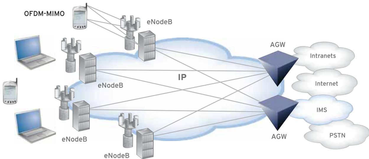
A typical LTE/SAE network will have two types of network elements supporting the user and control planes.
